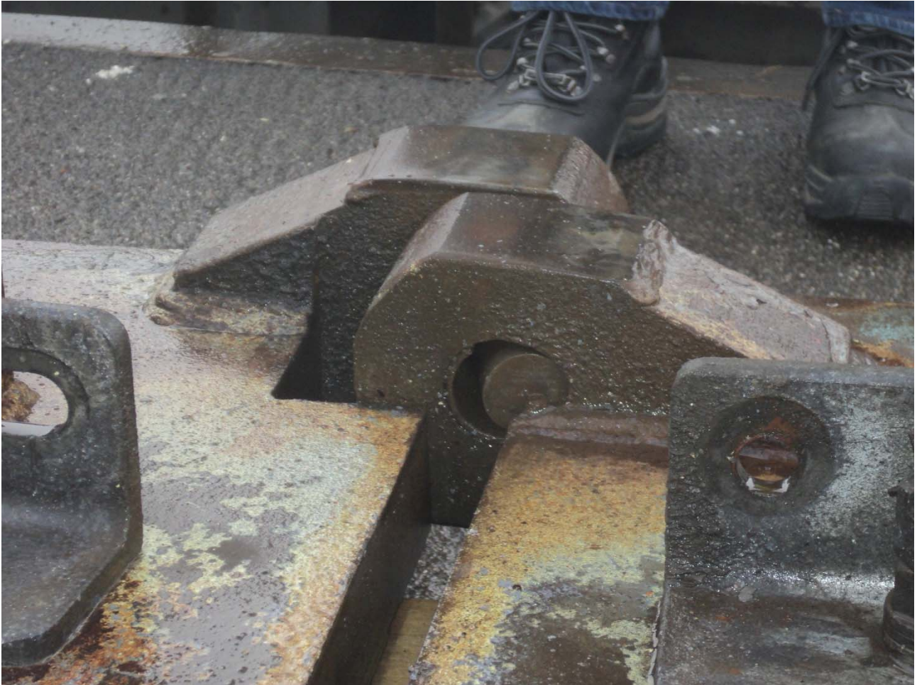
Photograph 4 – Note previous weld repairs to foot, now worn, and wear to hinge
