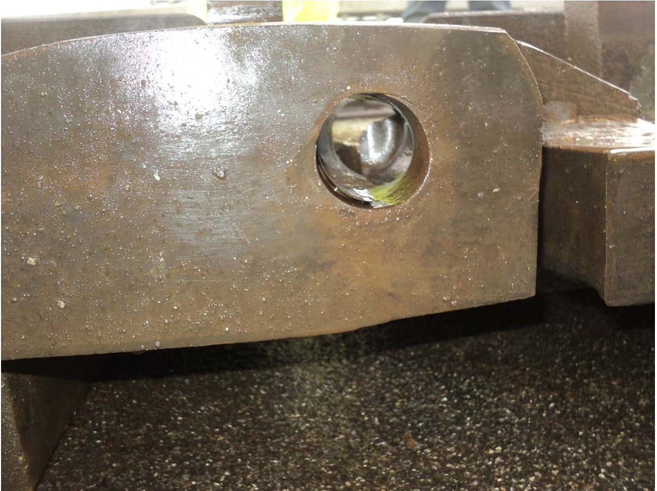
Photograph 5 – Worn and deformed pin hole. Bushing worn and loose. Worn foot profile.
