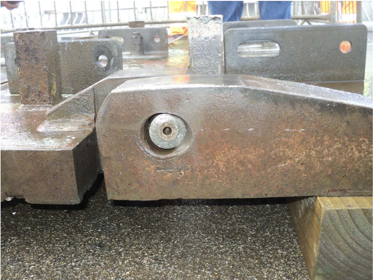
Photograph 12 – Excessive wear on foot and hinge
