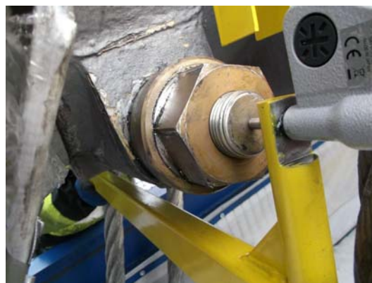
New bolt being measured
