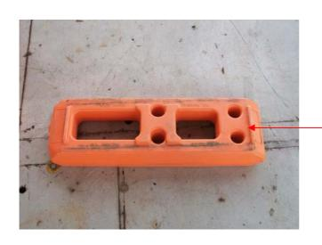
Weights used to carry out Static load test. 22 Kg.
