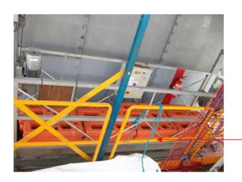
Static load test weights applied to feeder cradle, Total load applied as specified based on 22 Kg weights .
