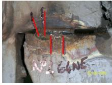
No.2 Stringer 64 N.E., only a small amount of weld actually holding packer to joint. These are indicated between the red lines.
