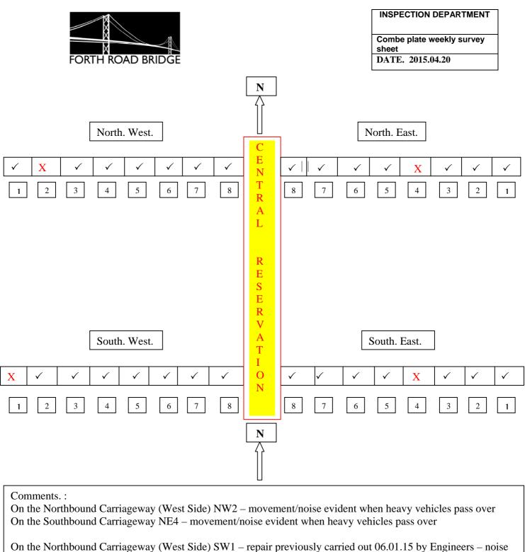
On the Northbound Carriageway (West Side) SW1 – repair previously carried out 06.01.15 by Engineers – noise was still evident on east side of SW1 - spring packs replaced on SW1 and SW2, further works to be carried out On the Southbound Carriageway SE4 – movement/noise evident when heavy vehicles pass over Southbound Carriageway SE2 – there is slight movement on the west side.
