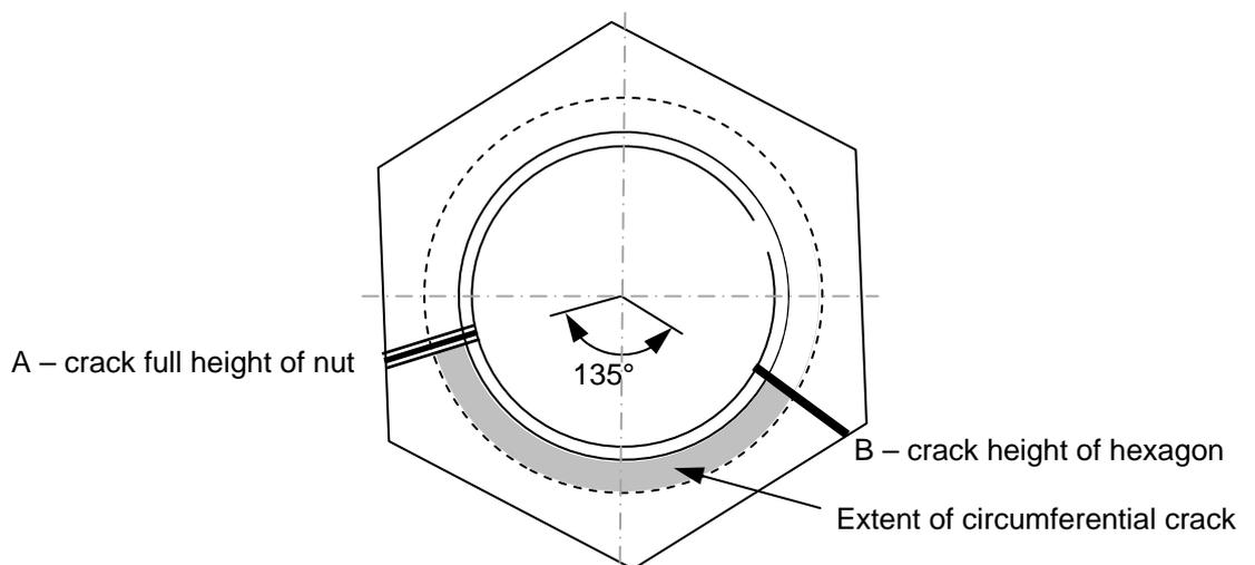
Fig 2.40: Plan layout of cracks
