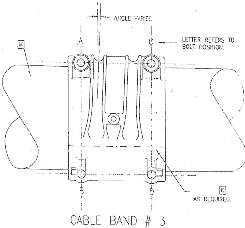
Cable band bolt A and B are the lowest set of bolts in a cable band.
