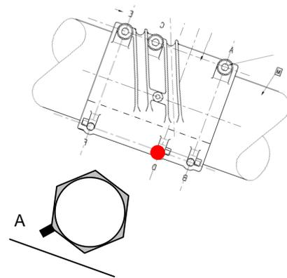
Fig 2.27: Location of nut and crack
