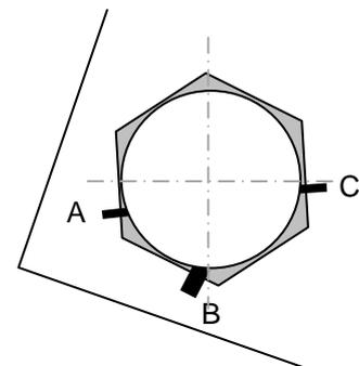
Fig 2.04: Location of cracks around nut
