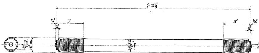
Fig 5.01: Original Bolt (from Drawing ACD2214 Rev. 3)
