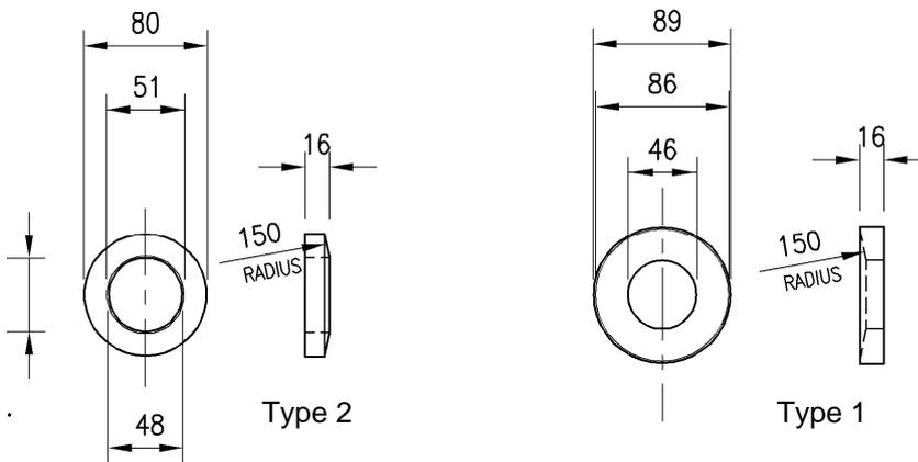
Fig 5.06: Replacement Washer – Dead End (from WAF 33111/AB/21)
