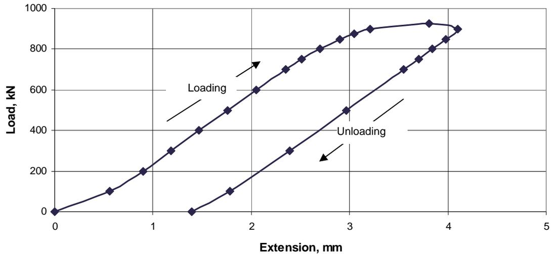
Fig 5.11: Load-extension curve for test 98HC357C (plotted from data)
