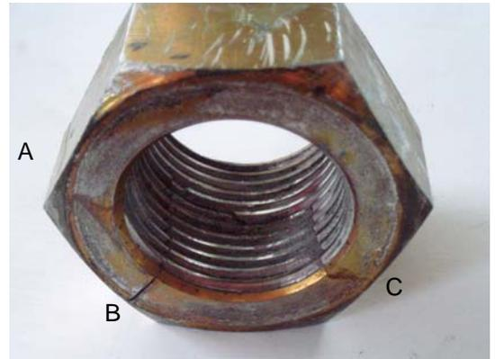
Fig 2.33: Cracks A, B and C
