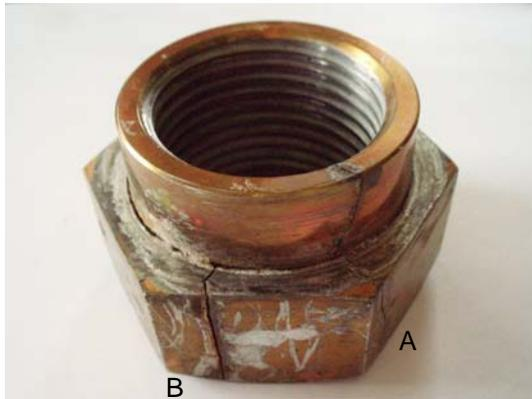
Fig 2.32: Cracks A and B
