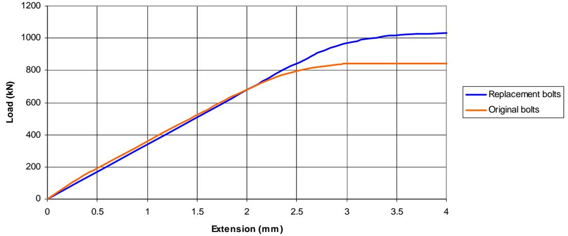
Fig 5.27: Comparison of Load-Extension curves for original and replacement bolts
