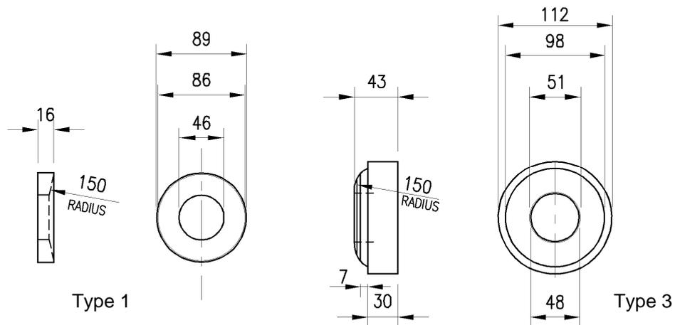
Fig 5.07: Replacement Washer – Live End (from WAF 33111/AB/21)
