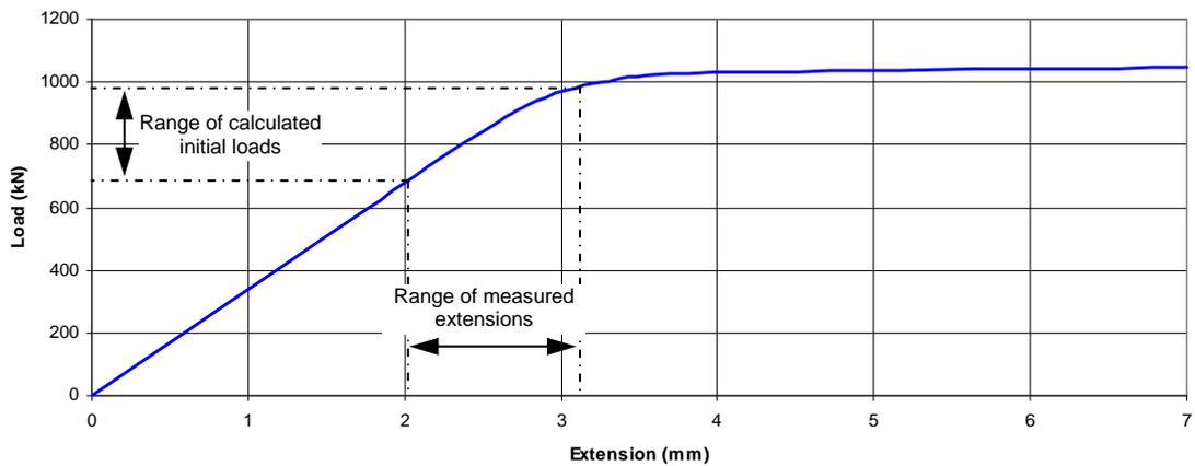
Fig 5.25: Estimated average load-extension relationship for replacement bolts
