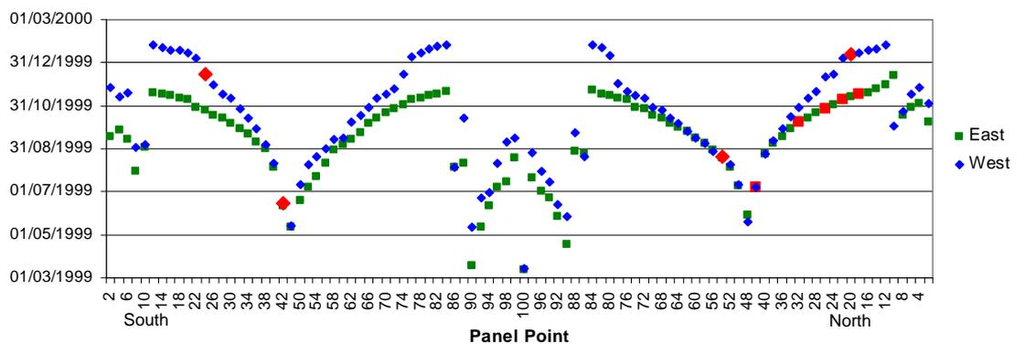
Fig 5.21: Bolt tensioning programme
