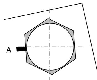
Fig 2.16: Location of cracks around nut
