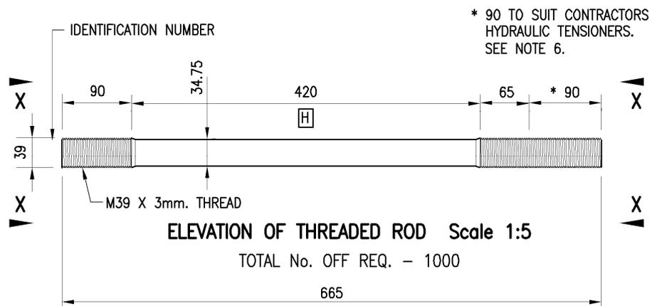
Fig 5.02: Replacement Bolt (from WAF Drawing 33111/AB/21)
