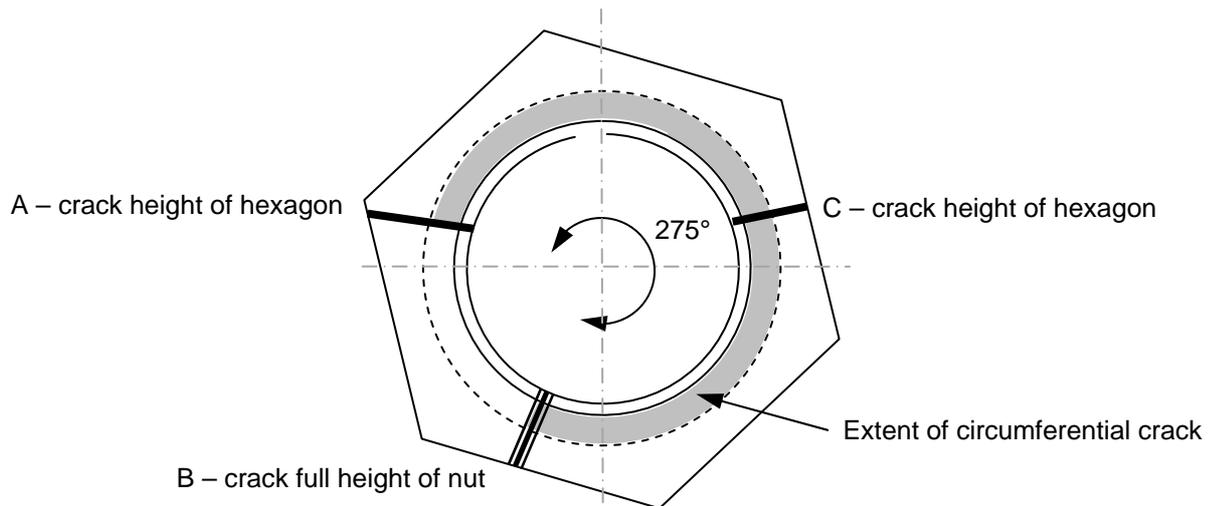
Fig 2.37: Plan layout of cracks
