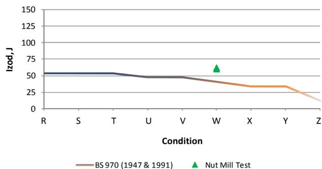
Fig 5.16: Izod Values – Replacement Nut Mill Tests and Specification
