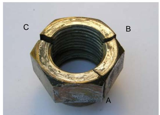
Fig 2.36: Cracks A, B and C
