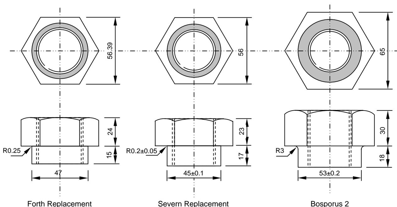
Fig 5.08: Comparison of nut sizes on various suspension bridges
