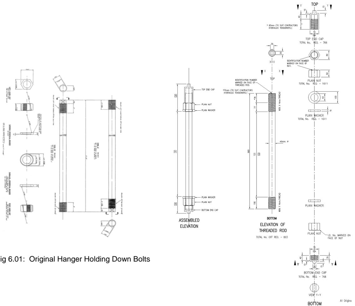
Fig 6.01: Original Hanger Holding Down Bolts
