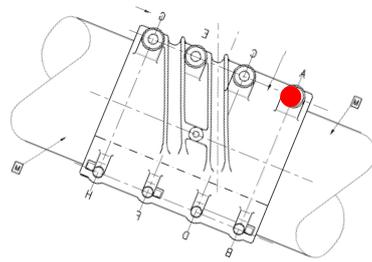
Fig 2.11: Location of failed nut on cable band
