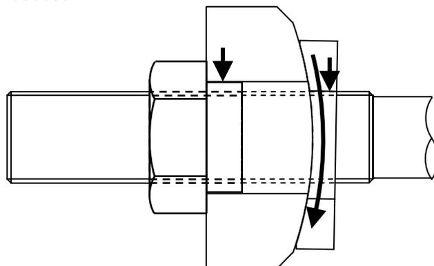
Fig 2.21: Slippage of live end washer under self weight
