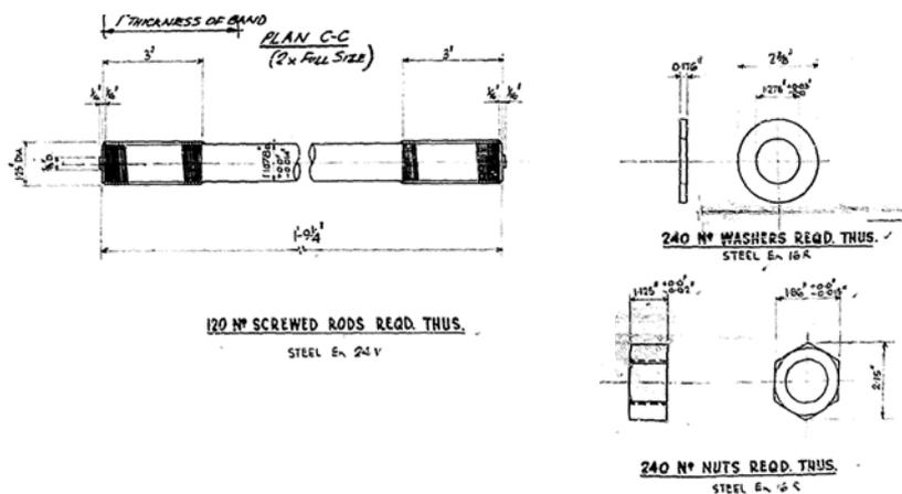
Fig 6.03: Back Stay Cable Band Bolts (ACD 2215)
