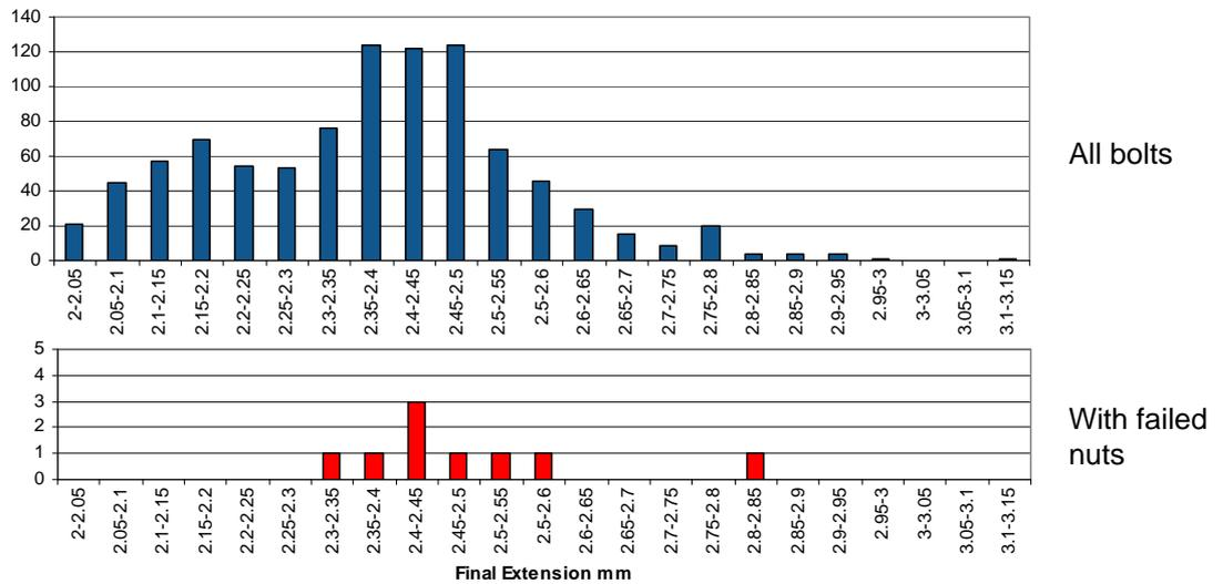
Fig 5.29: Distribution of Final Extensions from all bolts and those with failed nuts
