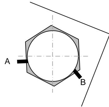
Fig 2.12: Location of cracks around nut
