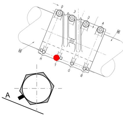
Fig 2.31: Location of nut and crack
