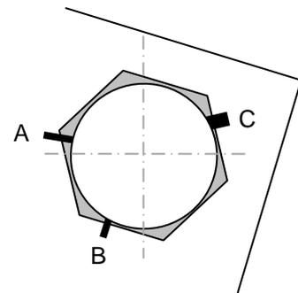
Fig 2.08: Location of cracks around nut
