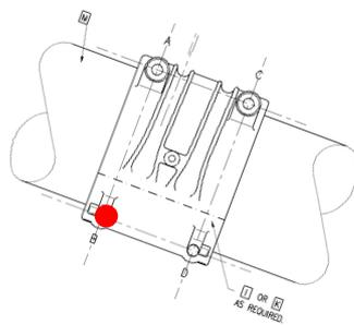
Fig 2.03: Location of failed nut on cable band
