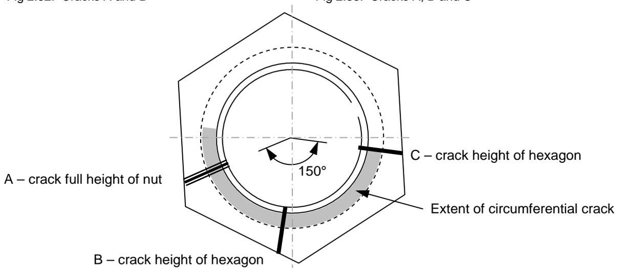
Fig 2.34: Plan layout of cracks
