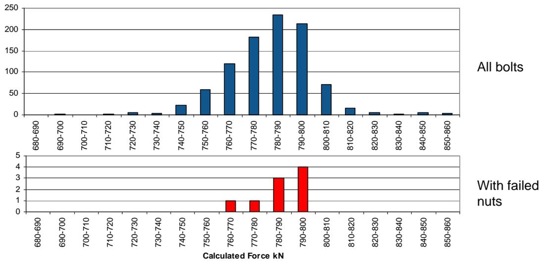
Fig 5.30: Distribution of Calculated Forces from all bolts and those with failed nuts
