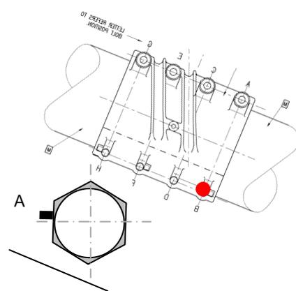
Fig 2.29: Location of nut and crack
