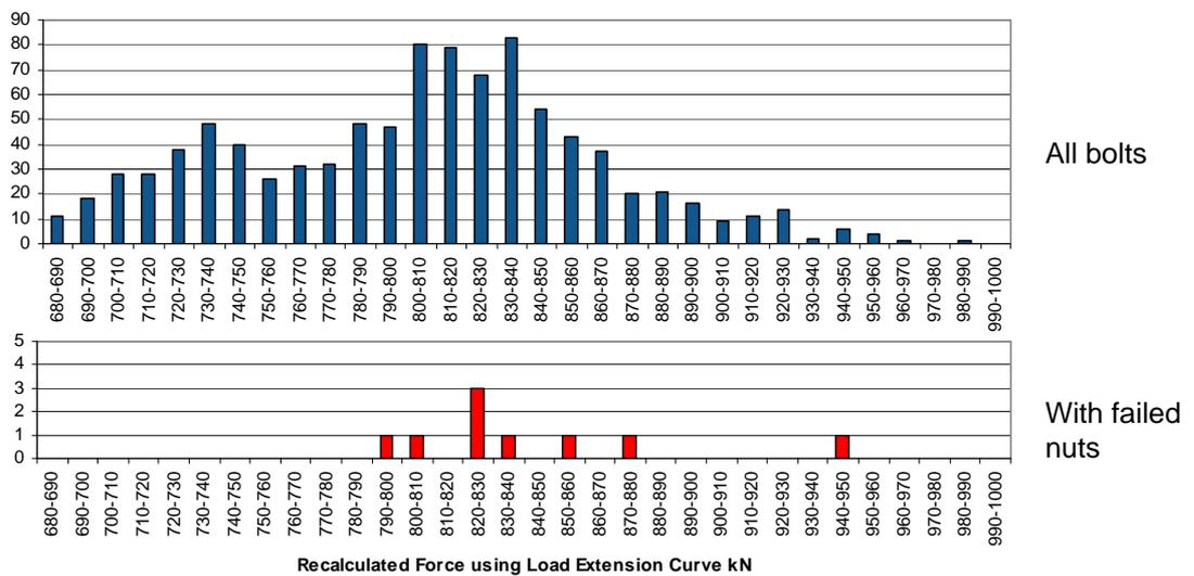
Fig 5.31: Distribution of Recalculated Forces using Load Extension Curve, from all bolts and those with failed nuts
