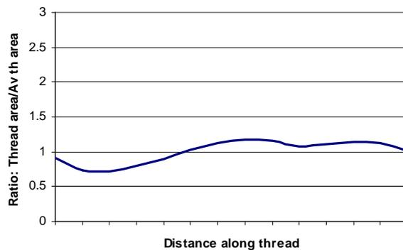
Fig 5.36: Calculated load distribution along thread helix for Roberts nut
