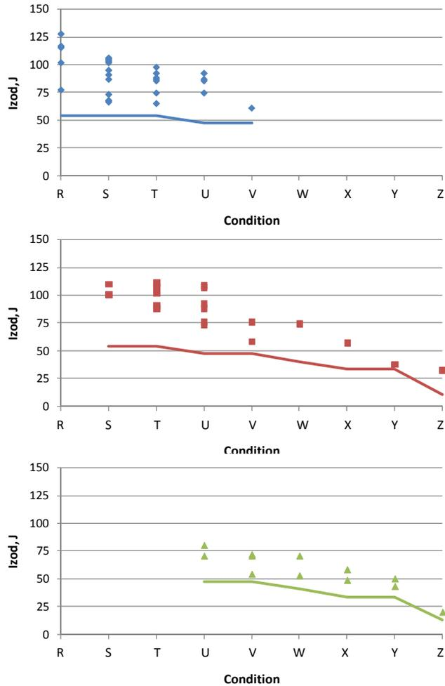
Fig 5.15: Izod values of steel samples, from BS 971:1950
