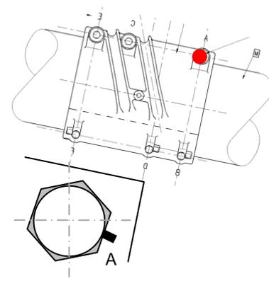
Fig 2.25: Location of nut and crack
