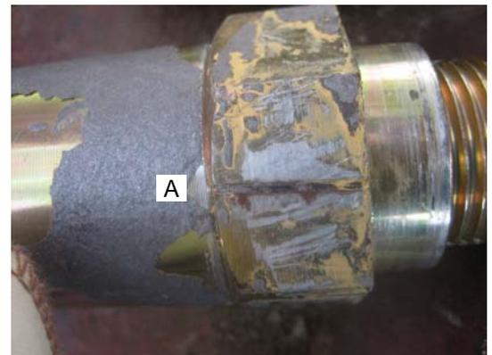
Fig 2.14: Crack A on removal, note paint in crack
