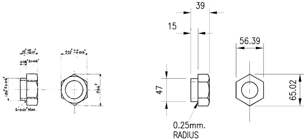
Fig 5.03: Original Nut (from ACD2214 Rev. 3) Fig 5.04: Replacement Nut (from WAF 33111/AB/21)
