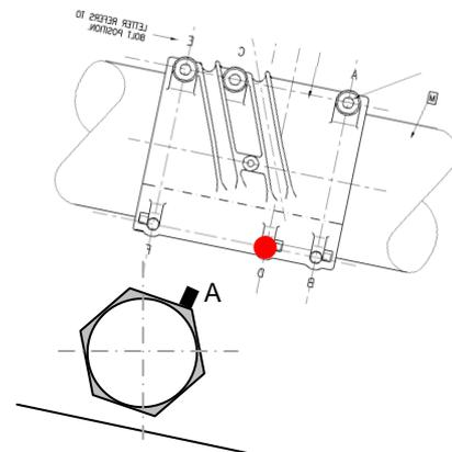
Fig 2.23: Location of nut and crack
