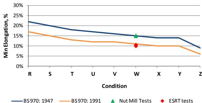
Fig 5.14: Comparison of Specified Minimum Elongations
