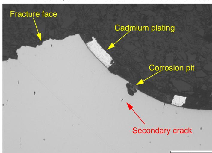
Fig 3.01: Metallurgical section at machined radius
