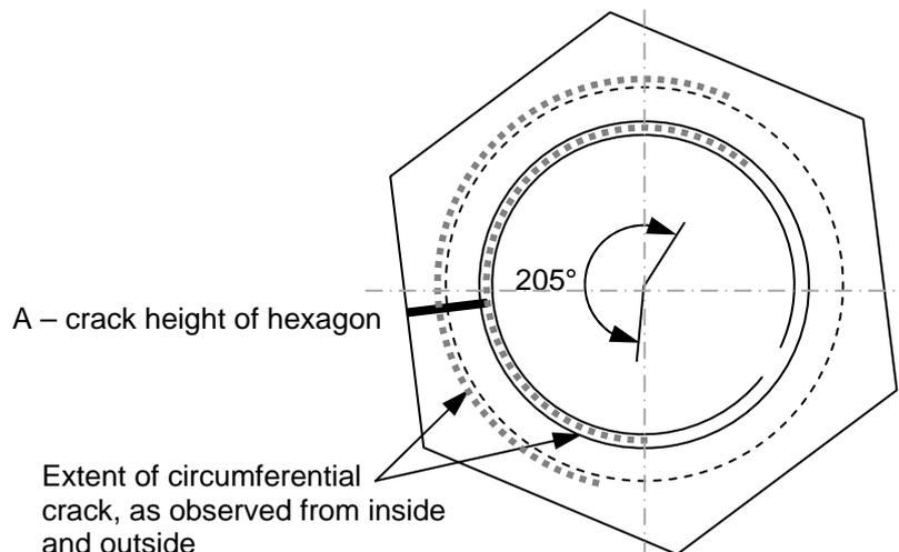
Fig 2.43: Plan layout of cracks
