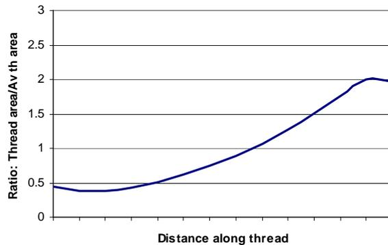
Fig 5.31: Calculated load distribution along thread helix for full normal nut
