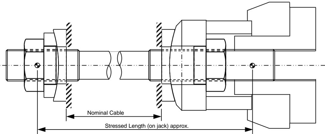
Fig 5.20: Bolt stressed length under jack
