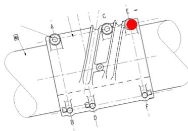
Fig 2.15: Location of failed nut on cable band
