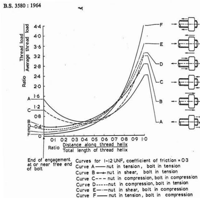
Fig 5.34: Theoretical load distribution along thread helix
