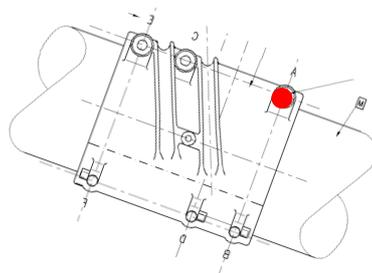
Fig 2.07: Location of failed nut on cable band
