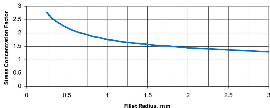
Fig 5.32: Calculated stress concentration factor at re-entrant corner (from Roark & Young)
