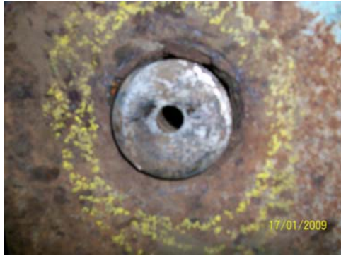
Position No. 8 External: Protruding pin, seized on inner lug. Pin ground down to ease reinstatement.
