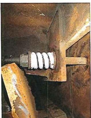
New springs fitted to tongue plate
