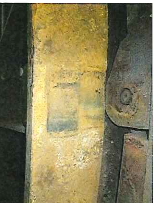
Example of Wear to Radius Arm from Bushes
