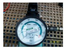
Pressure taken up to 19,000 psi. this procedure was carried out a further two times as specified.
