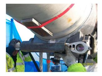
Prior to leaving platform photographs & dimensions were taken on the gaps between the nut size against the cassette contained in the RSL 6 as it was found that the required movement was to much before a reaction point was reached to allow the tool to bite. Discussions between Maintenance manager took place that evening to design and fabricate this insert which would be used to counteract excess movement .
