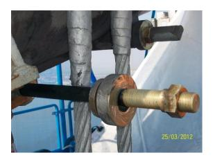
14.30. PM. Bolt torqued up using the RSL. 6. New bolt readings were taken and recorded on Bolt scan EMS., machine 184 group 1 under bolt No 21. New bolt "L "referenced AT 660.084.
