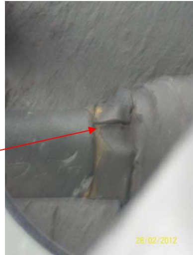
PP. 24. Bolt "D" Dead side nut, crack recorded. On top & bottom faces of nut.
