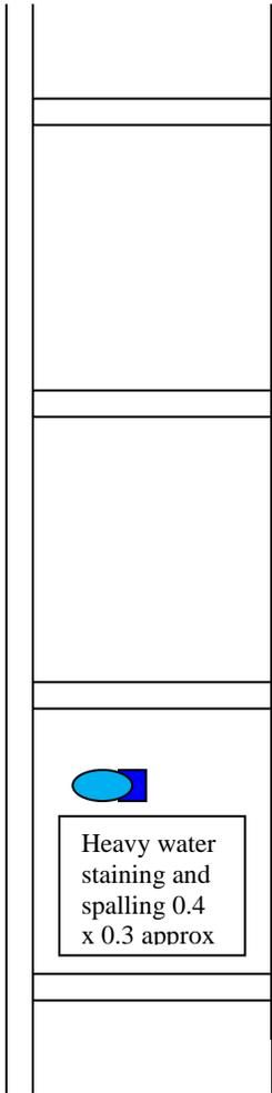
Heavy water staining and spalling 0.4 x 0.3 approx
