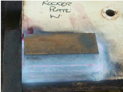
SE3. END BEARING BLOCK ON ROCKER PLATE (E) TESTED & INSPECTED
