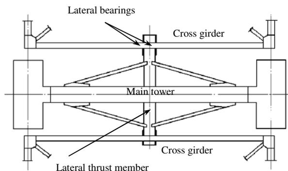
Figure 2 – Arrangement of Lateral Bearings at Main Towers
