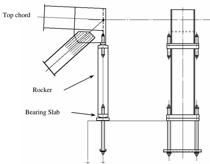
Figure 3 – Arrangement of Rockers at Side Towers
