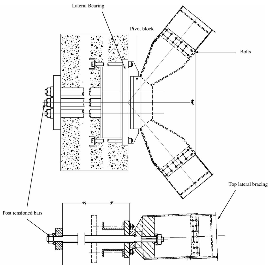
Figure 4 – Arrangement of Lateral Bearings at Side Towers
