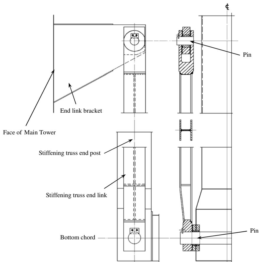
Figure 1 – Stiffening Truss End Link
